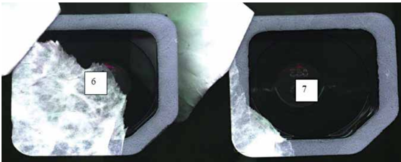
Figure 20. Results of improper lid placement during DuPont sealing experiment.
