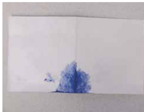
Figure 16. Wicking occurs when dye is left too long in the pouch during ASTM F1929:2003 testing.
