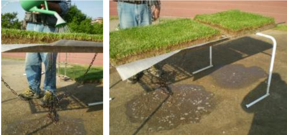
Tests done on a scale model before the installing the natural grass. The test was done in order to assess the precise permeability performance of DuPont™ Typar®; photographs by Bruno Marabotto, all rights reserved.
