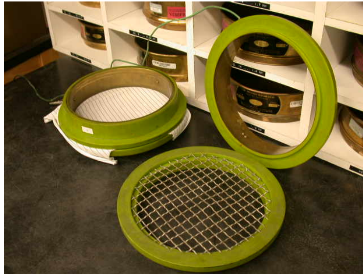
Figure 1: AOS specimen holder, of the size of a standard 8" sieve
